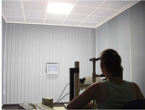
Figure 5 – Subject in test room during task 1. The subject firstly calculates the row results and secondly subtracts the smaller value from the bigger value.
