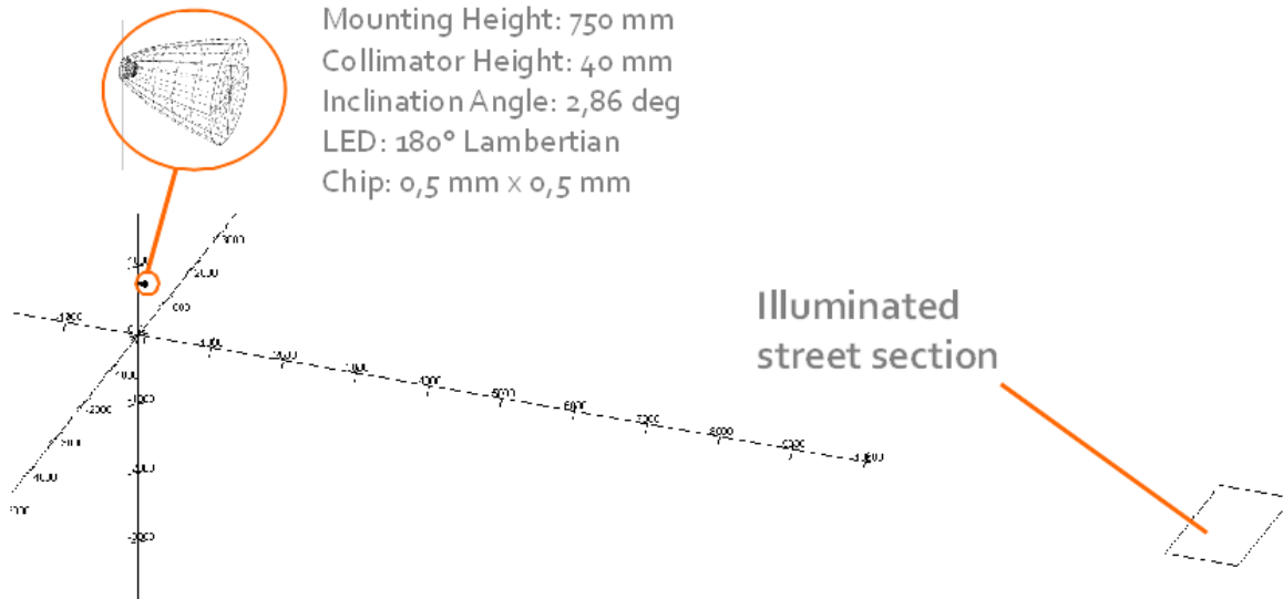
Abbildung 6: Setup LucidShape, LED Kollimator
